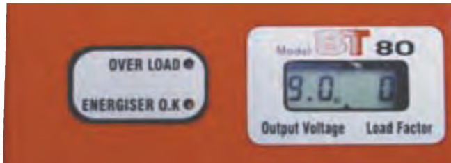
BT80 Energiser showing LED display
